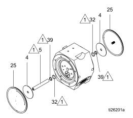
12. Lubricate the shaft, then install it in the air motor assembly (2). Turn the diaphragm as you push it in. Then, tighten the other diaphragm onto the shaft, hand tight only.
