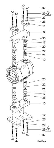
8. Align the outlet manifold (8) on the assembly with the outlet port facing in the correct direction for your application.
