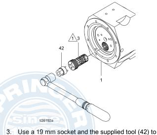
. Use a 19 mm socket and the supplied tool (42) to tighten the spool assembly (3) until it is flush with surface of the air motor assembly.
