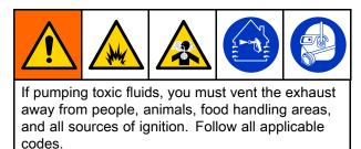
**NOTE:** Do not restrict the air exhaust port. Excessive exhaust restriction can cause erratic pump operation.
