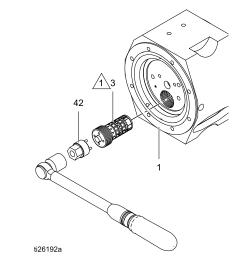
Inspect each spool assembly (3) for worn or damaged parts. Replace each assembly as needed.
