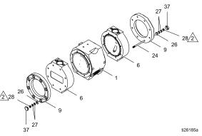
37 10. Remove the nuts (28) and bolts (24) by using two 10 mm wrenches, to hold on one side and to turn the other. The nuts (28) will come off of one side only. Remove the bolts (24).
