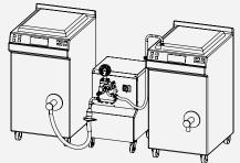
When the product in the first pasteurizer reaches the pasteurization temperature of 85-90°C, then the homogenizer transfers the product into the second pasteurizer to accomplish the cooling duty.
