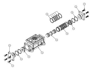
**Valve Assembly for Aluminum Mid Sections**
