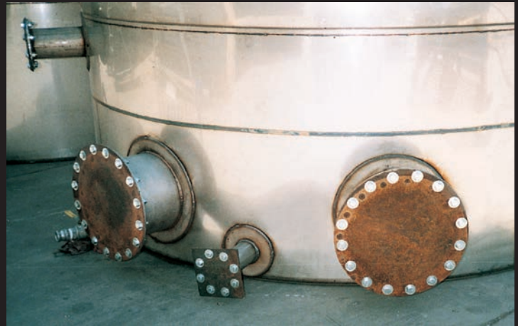
All fittings are mounted in hydraulically extruded nozzles for strength.
