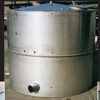
Bottoms and tops have full radius rolled corners for reduced weld distortion and ease of cleaning.
